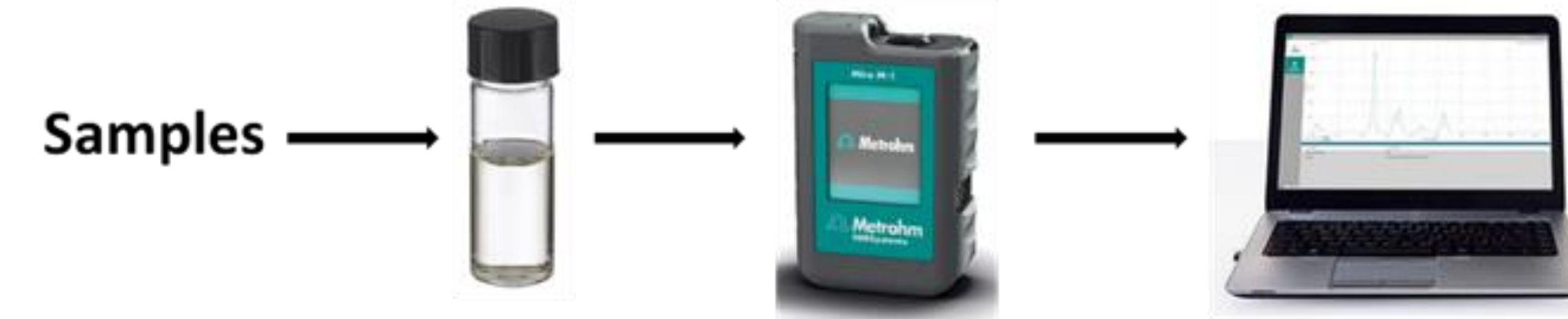
Figure 2b: A schematic diagram that displays the overall method of RS using Mira M-1 device and RS analysis with MiraCal software (Metrohm, USA)
